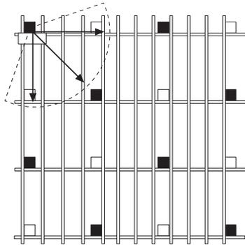
First, locate the embedded tubes in the columns where the Fall Arrest System is going to be accommodated and then begin the boarding process from that point.
