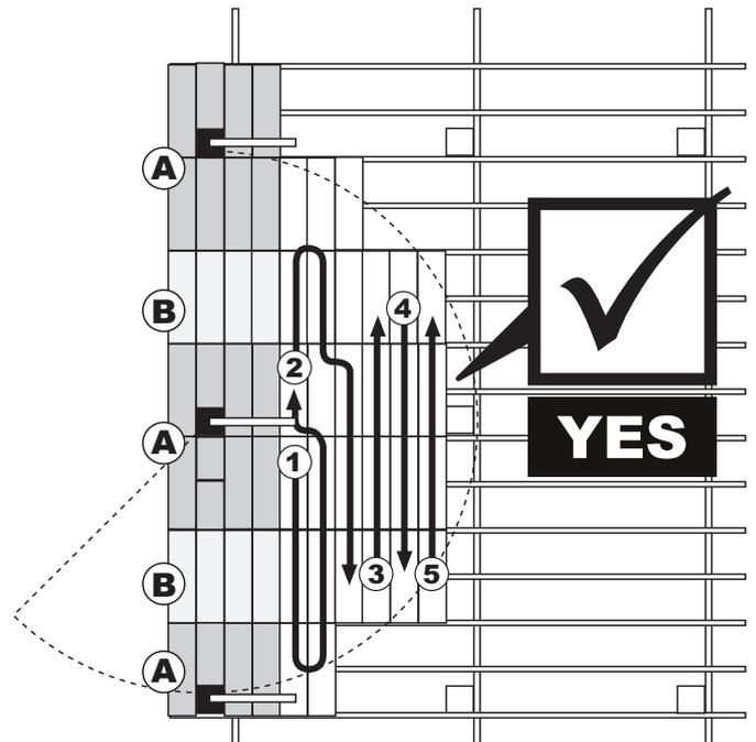
By replacing the Retractable Element (8441201 / 84439) and the Harness Lengthener (84423 / 84474) with a Fall Arrest Block (EN360 Compliance) of 6.5 m, or combination of 6 m + 0.5 m extender, the user can increase the distance forward from the Alsipercha body that is protected.
