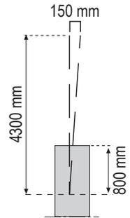
(\* ) This tolerance will vary depending on the column section. If using the Alsipercha system in columns with a section smaller than 30 cm, cracks may appear in the concrete. In this case, consult the structure client.
