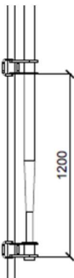
Once the two Ring lock adapter (83078) and the column clamp sleeve (83426) are installed, insert an Alsipercha (84411 / 83471) unit; start installing in the central hole of the Ring lock adapter in the upper position, and then pass it through the central hole of the Ring lock adapter in the lower position. Ensure that the lower part of the ALSIPERCHA is correctly and completely inserted, until it reaches the bottom, internal part of the column clamp sleeve (83426).
