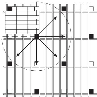
Then begin the boarding process from one end of the surface and work safely with a radius of 6.5 m, which equals approximately 125 m<sup>2</sup>.
