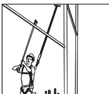
Use the hook to do this if the next Alsipercha is positioned so that the worker cannot reach to anchor themselves.
