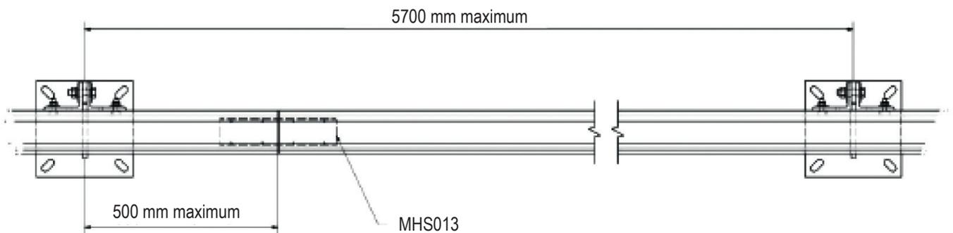
Fig. 7 – Distance between joint and **Alsipercha**
