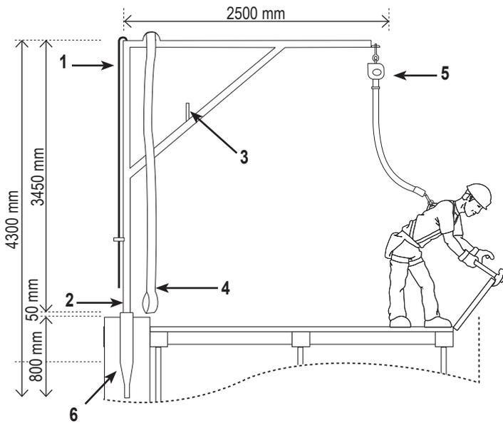
**Technical details for arranging the housing tube. Housing tube tolerances.**
