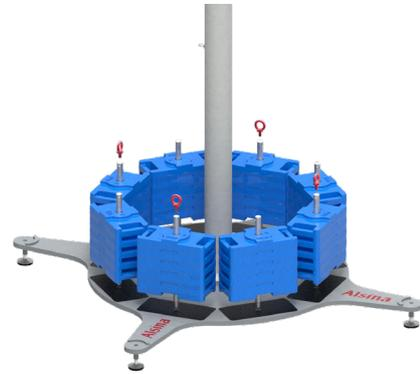
Fig. 8. Positioning the counterweights
